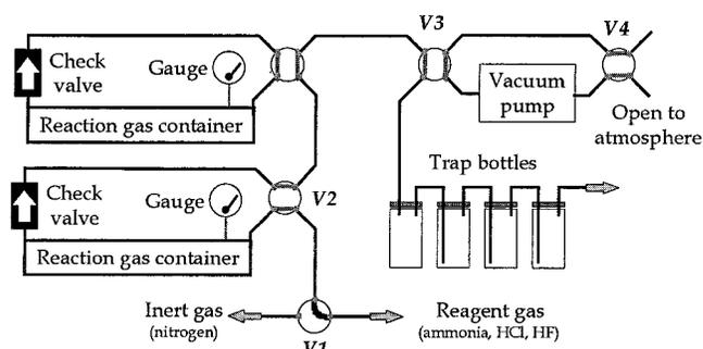
**Figure 3.** Apparatus with vacuum compatible reaction gas container.
